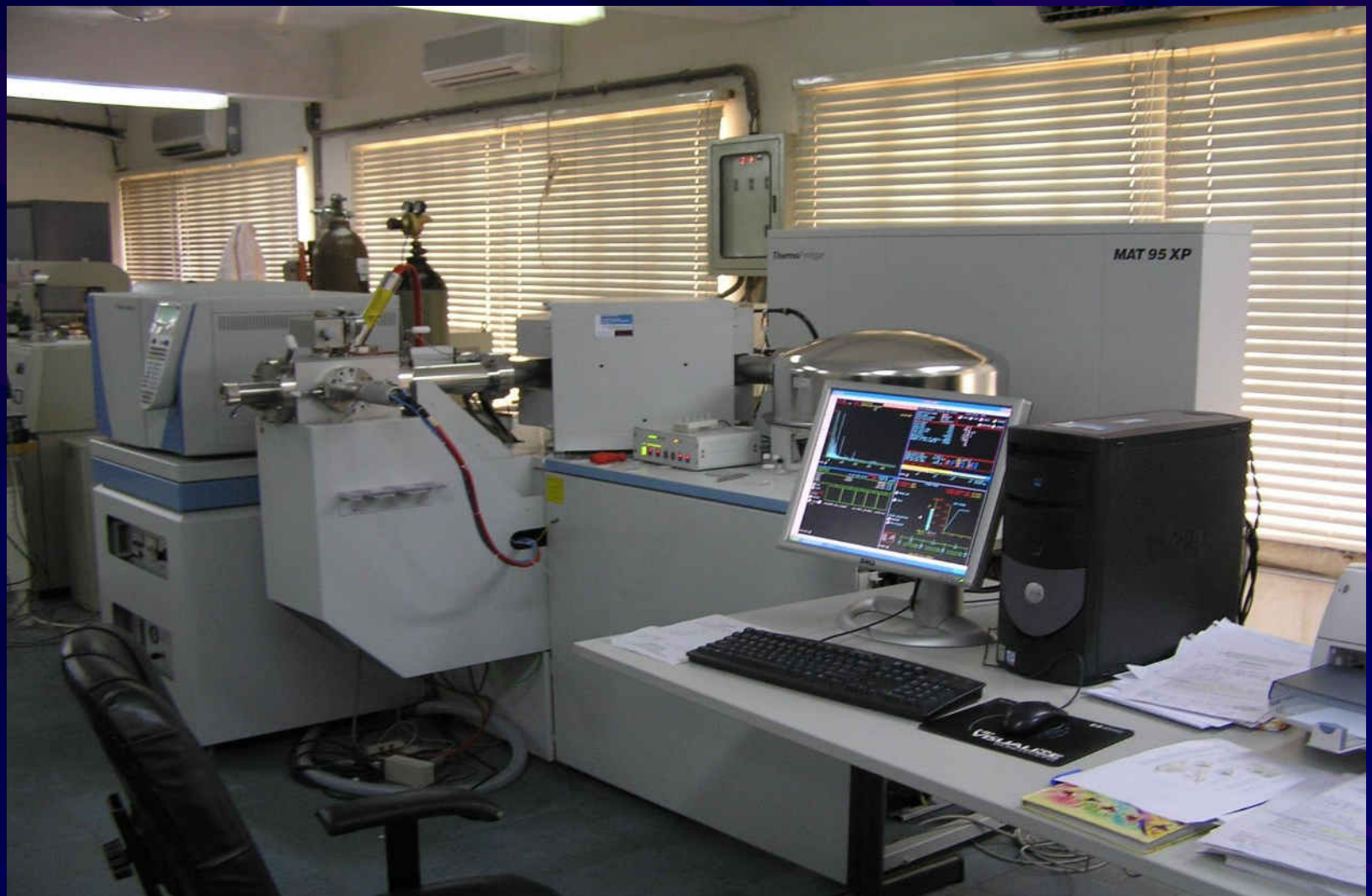
MASS SPECTROMETER (ELECTRON BOMBARDMENT SYSTEM)
